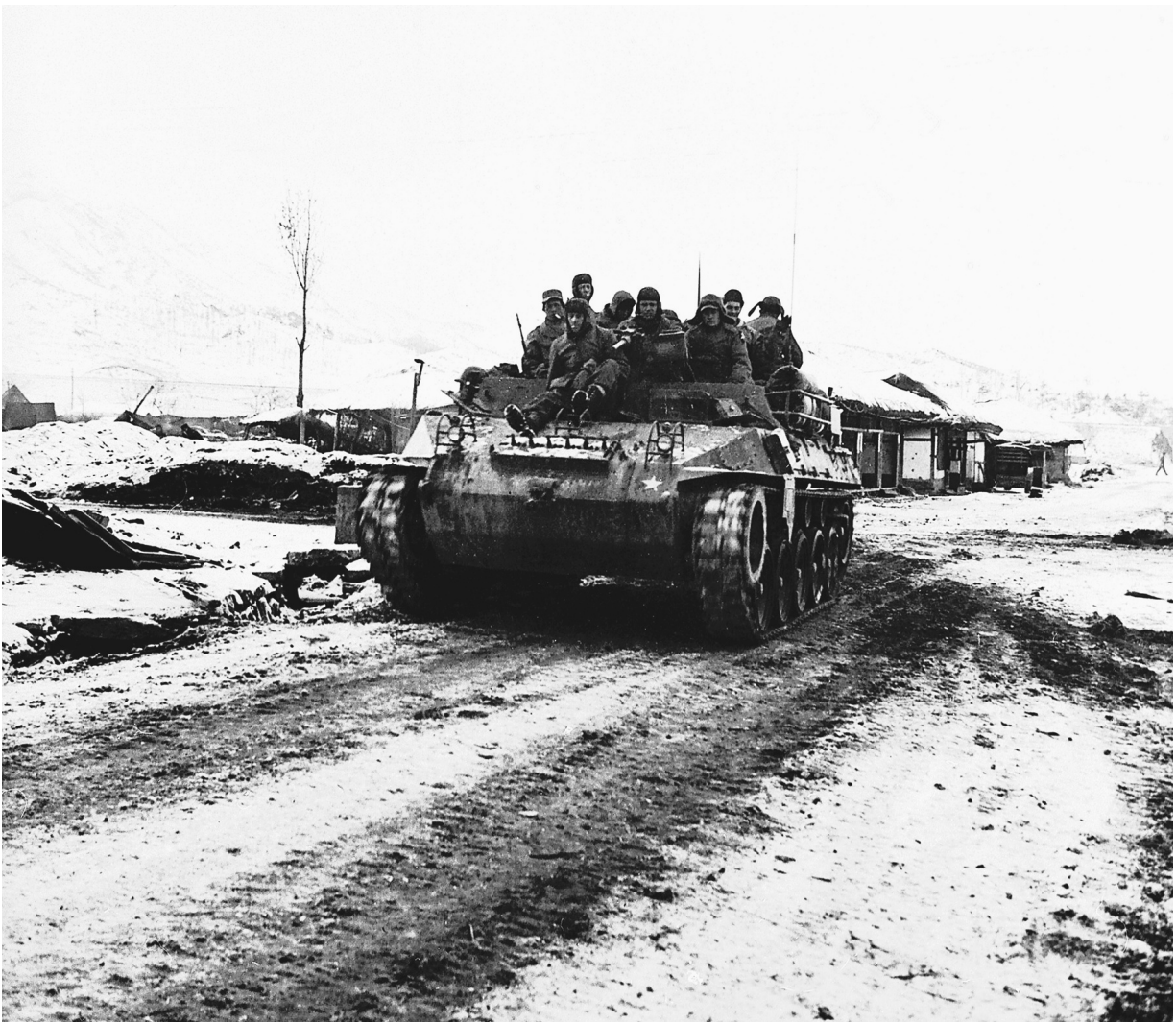
Soldiers from the 2nd Infantry Division's reconnaissance company ride in an M39 armored utility vehicle, which came into service at the end of World War II and used the same chassis as the M18 Hellcat tank destroyer. This photo was taken on February 10, 1951. REAL WAR PHOTOS
