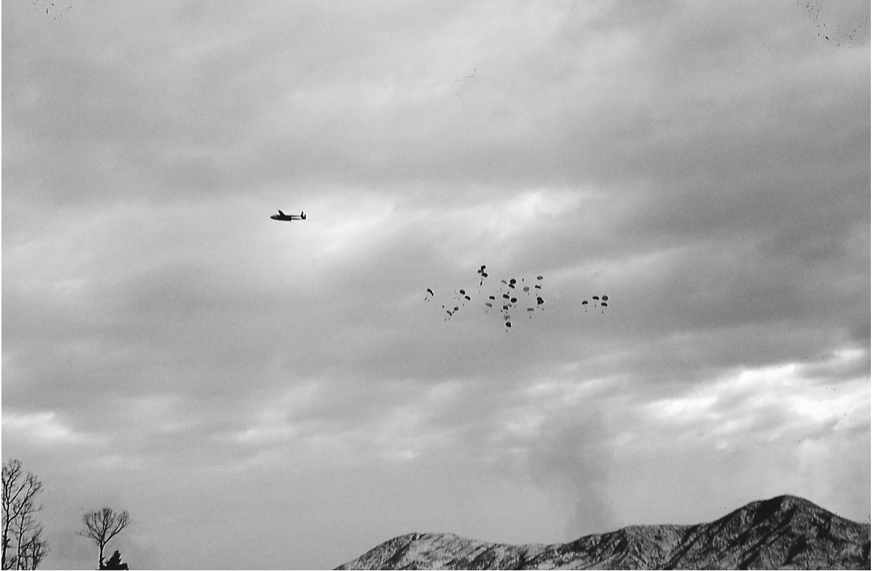
A C-119 Flying Boxcar over Chipyeong-ni. With the Chinese surrounding it, the only way the 23rd Infantry could receive supplies was through air drops. The standard C-119 could carry over 20,000 pounds of supplies. LT. COL. KINGSTON WINGET
