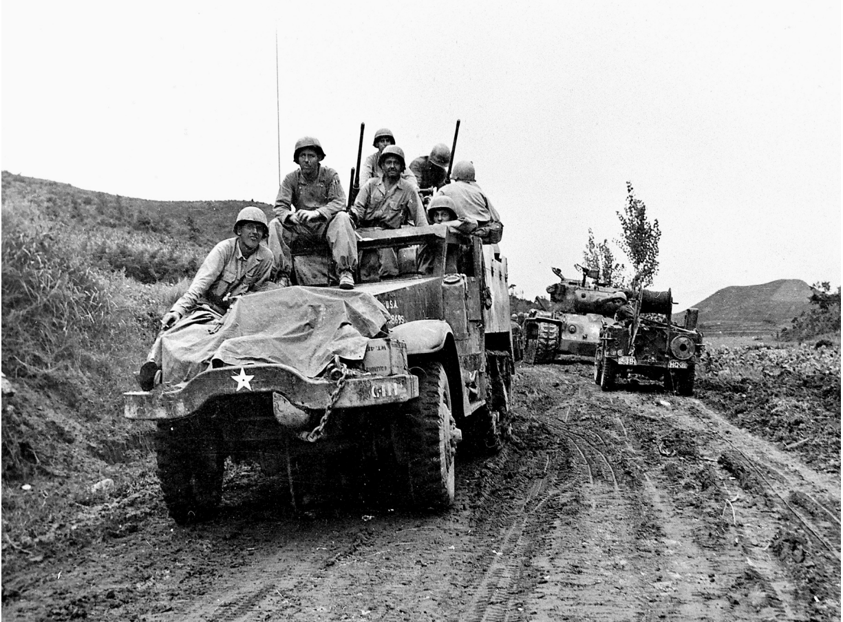
An M16 half-track from B Battery, 82nd Antiaircraft Artillery Automatic Weapons Battalion, mounting four .50-caliber machine guns on a rotating turret. B Battery used these weapons at Chipyeong-ni with deadly effect against the Chinese infantry. REAL WAR PHOTOS
