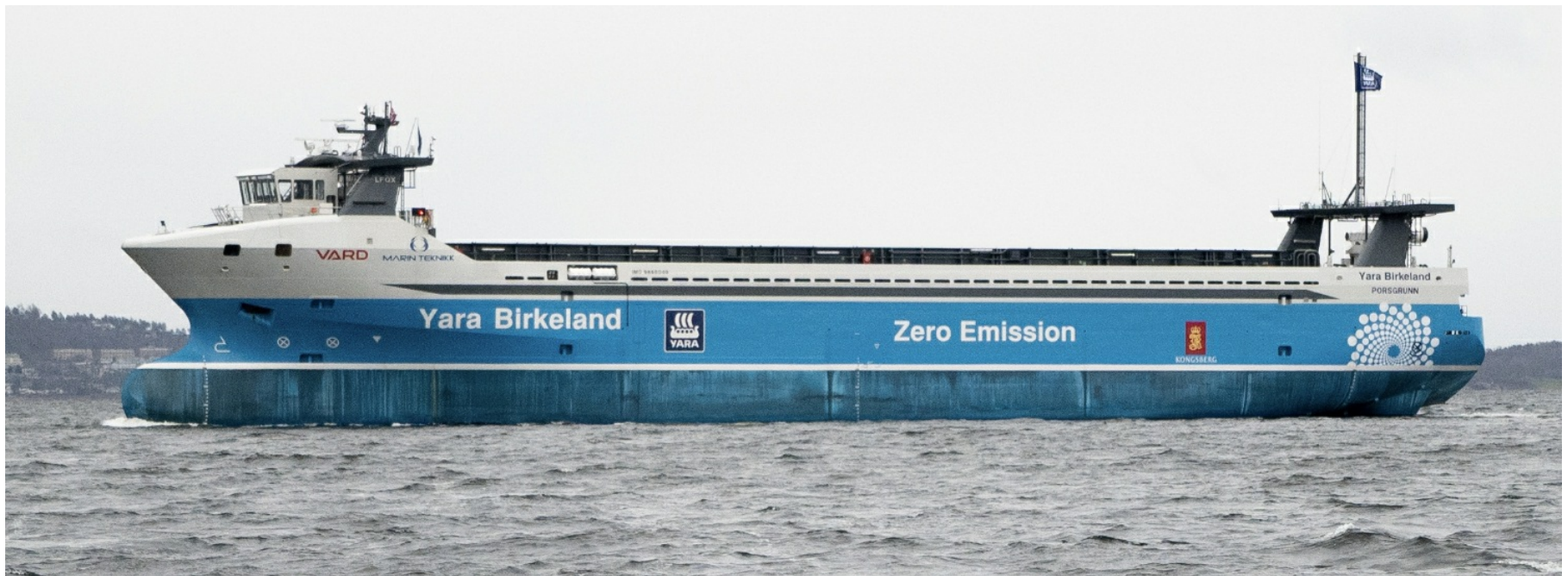
Figure 7.4. Autonomous, electric containership YARA BIRKELAND.
