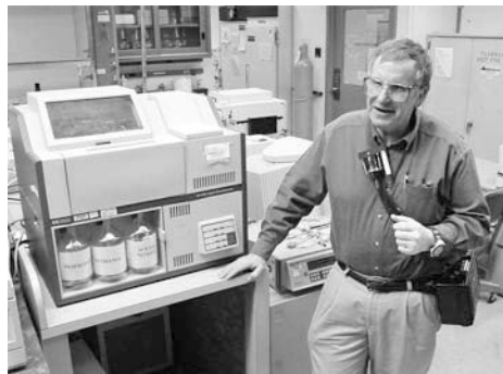
FIGURE 6.1 Air sampler used in the Sixteen Cities Study.
